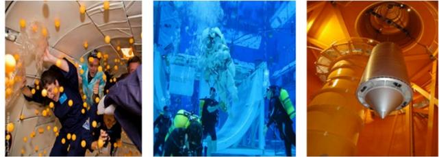
**Figure 2. Methods to simulate low-gravity conditions include use of parabolic flight (left), neutral buoyancy in large water tanks (center) and use of drop towers (right).**
