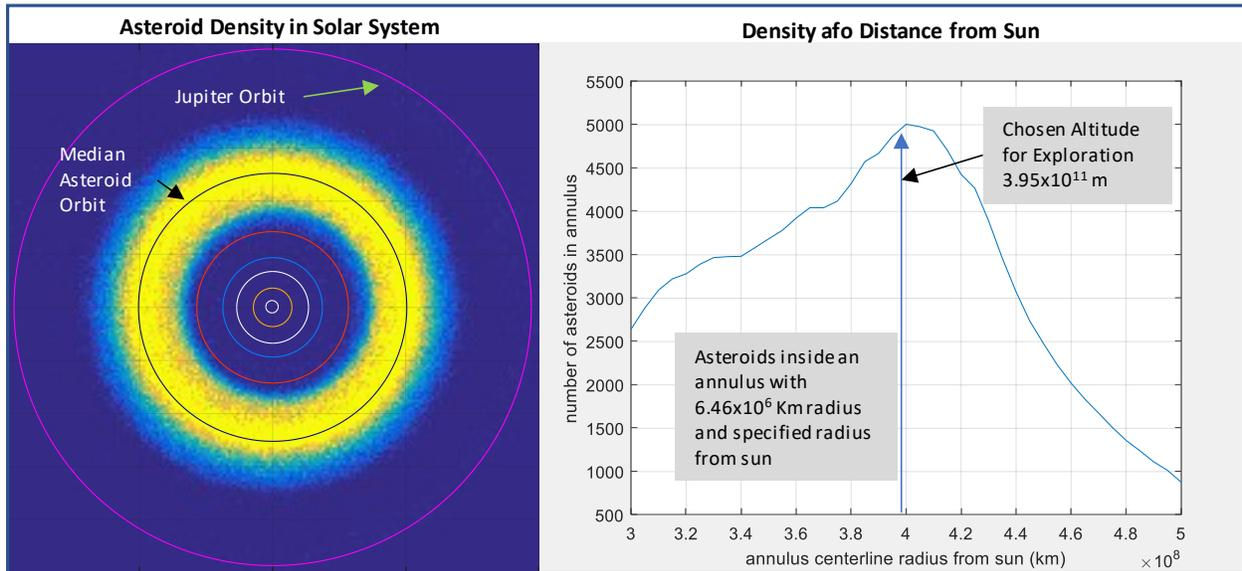
**Figure 3.** Nominal Mothership orbit is placed at the location of highest asteroid density
