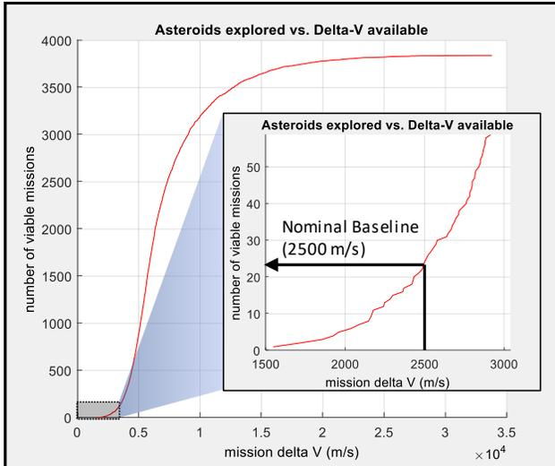
**Figure 6.** Number of viable missions rise quickly as nano-spacecraft delta-V increases above 2000m/s
