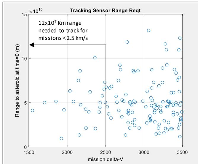
**Figure 8.** If Mothership must track asteroid Nano-spacecraft launch, about 120 million kilometers of range is required.
