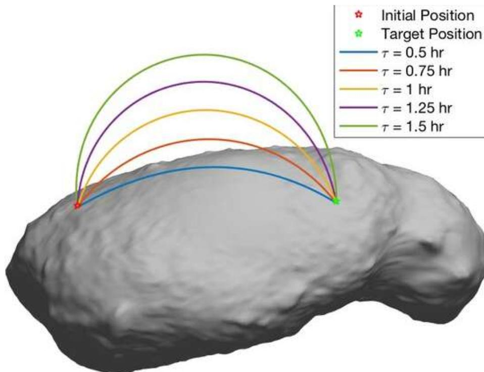
Hopping Trajectories from initial location to a target location on the surface of Itokawa. Credit: Kalita & Thangavelautham.
